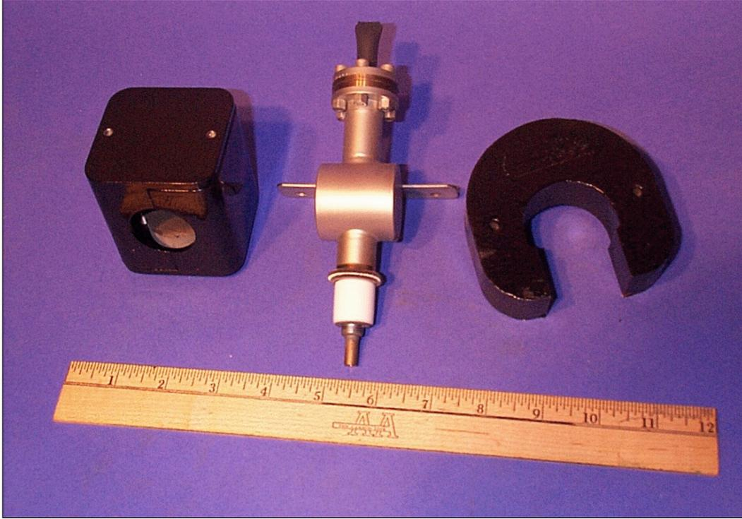
Figure 11: Varian style 2 liter per second pump with SmCo and Alnico 5 Magnets
