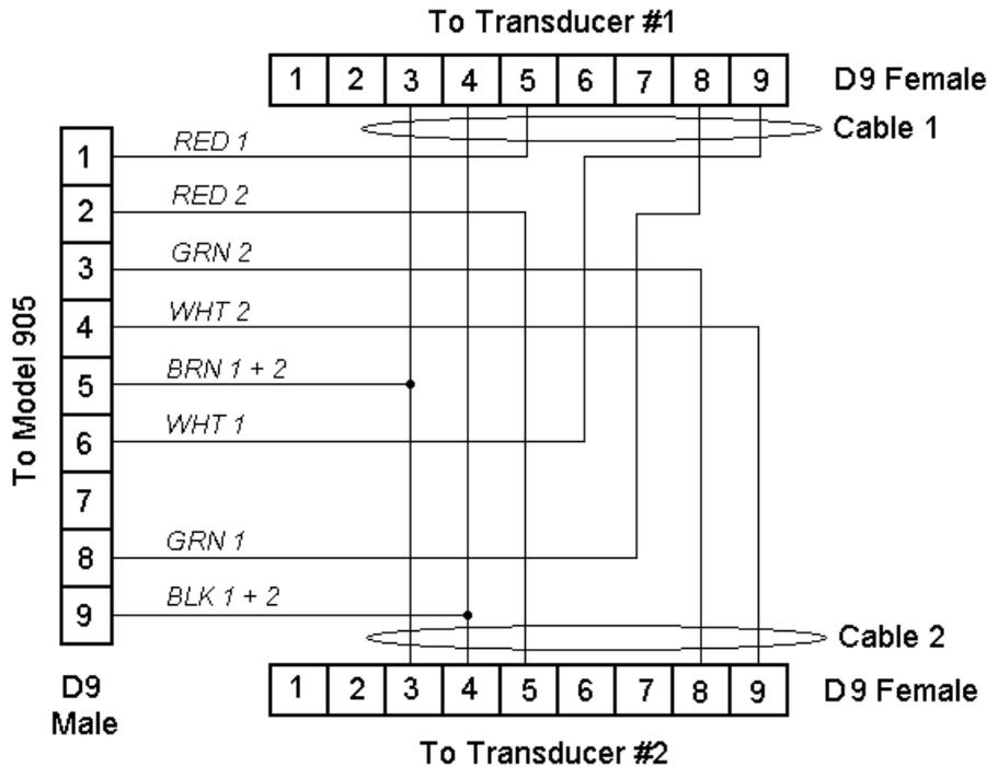
Fig. 7. Schematic for the Model 905 Sensor Cable (8100-900-10)
