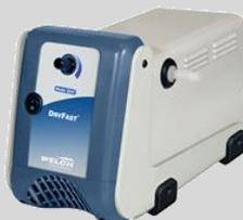
DryFast Research Chemical Duty Dry Vacuum Pump, 25 LPM x 29.7" Hg vacuum. Use vacuum regulator to control vacuum so you don't boil ("bump") solvent; "tune" to fastest solvent removal rate ("stripping rate"). This unit's deeper vacuum means you can strip even water at 77°F (25 °C)
