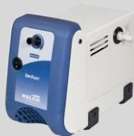
DryFast Collegiate Chemical Duty Dry Vacuum Pump, 35 LPM x 28.3" Hg vacuum. Use vacuum regulator to control vacuum so you don't boil ("bump") solvent; "tune" to fastest solvent removal rate ("stripping rate"). This unit is sufficient to strip Ethanol at bath temperatures of 95°F (35 °C)
