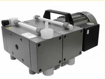
Chemical Duty Dry Vacuum Pump, 2.3 CFM x 29.86" Hg vacuum, 115v/60hz. Ideal flow rate and vacuum level for rapid purging that does not remove desired oil fractions. Use 331030-5 hose.
