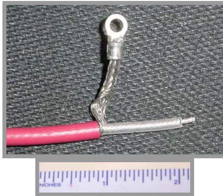
Figure 2 – HV Cable Prep Through Step 4
