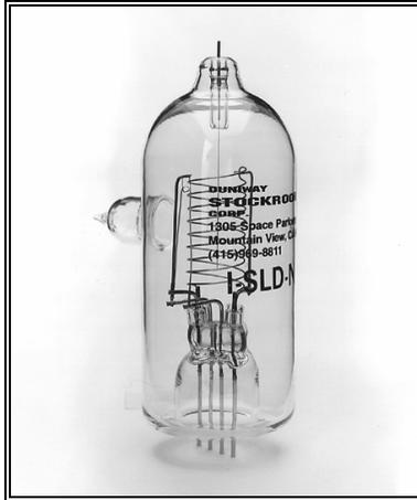
Glass Ionization Gauge - Sealed Reference Tube
