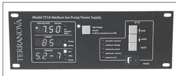
2. As the voltage rises toward 7.5KV (7500 volts), the current pressure display will fluctuate and you should hear a "sizzling" or "tickling" sound from the ion pump due to high voltage breakdown inside the pump.
