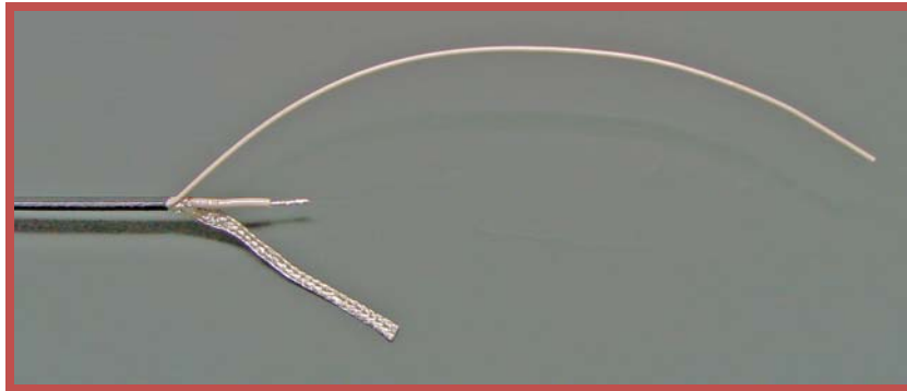
Figure 2: Prepare High Voltage Cable End as Shown Above Mesh Shield Length – 2.5 Inches Insulated HV Lead Length – 1 Inch Ground Wire Length – 8 Inches
